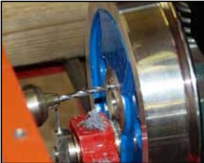
Centre Left: Pinning a wheel and checking the axle alignment with the coupling rods. Centre Right: Disc brake assembly. Bottom Left: Prime mover mounted on chassis. Bottom Right: First test of the chassis under power.
