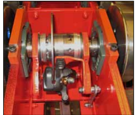
Centre Left: Pinning a wheel and checking the axle alignment with the coupling rods. Centre Right: Disc brake assembly. Bottom Left: Prime mover mounted on chassis. Bottom Right: First test of the chassis under power.
