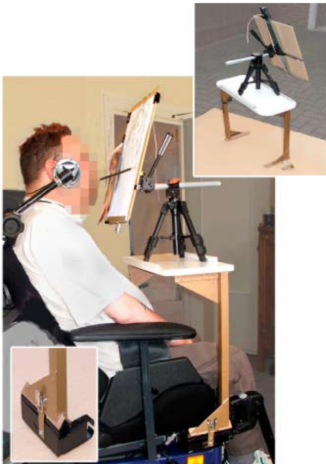
Left: This multi-axis drawing stand for a quadriplegic artist illustrates what can be done with simple items.
