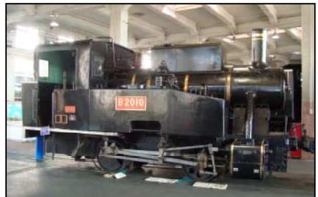
**Small goods locomotive built in Britain and used for moving coal**
