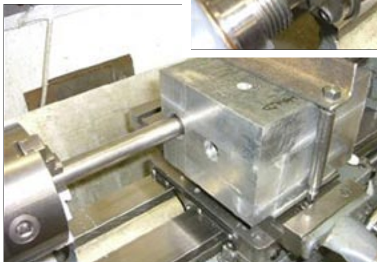
◀ Boring the holes for the camshaft with a boring bar
