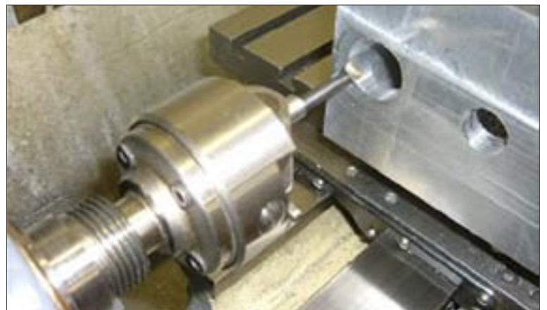
◀ Sizing the hole with a boring head
