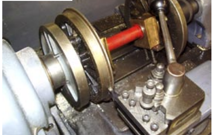
(Top right) Wheel profile at four times full size. (Top left) Wheel measurements. (Above) Plasticine impression of one of Speedy's wheels. (Right) Wheelset in lathe set to turn coned tread.
